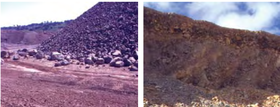
Figure 10: Base rubble zone (left image); angle of repose and trafficked layers (right image)
