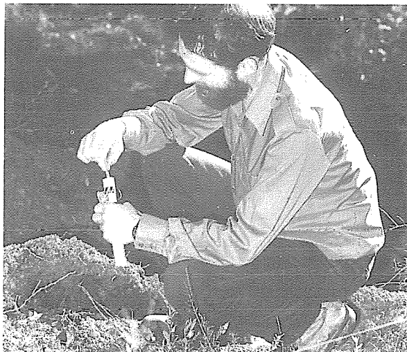
John Watt, loading a hole for weathering spread seismic refraction survey, to investigate spillway site for North Dandalup dam site.
