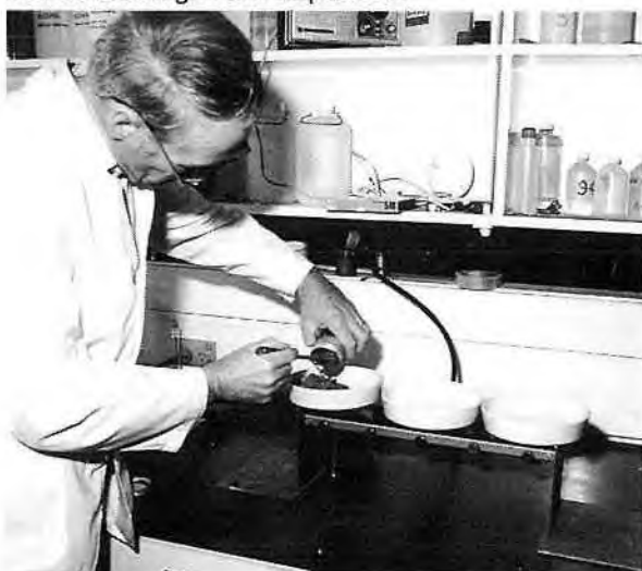
Investigating soil chemistry; preparation of saturation extract.
