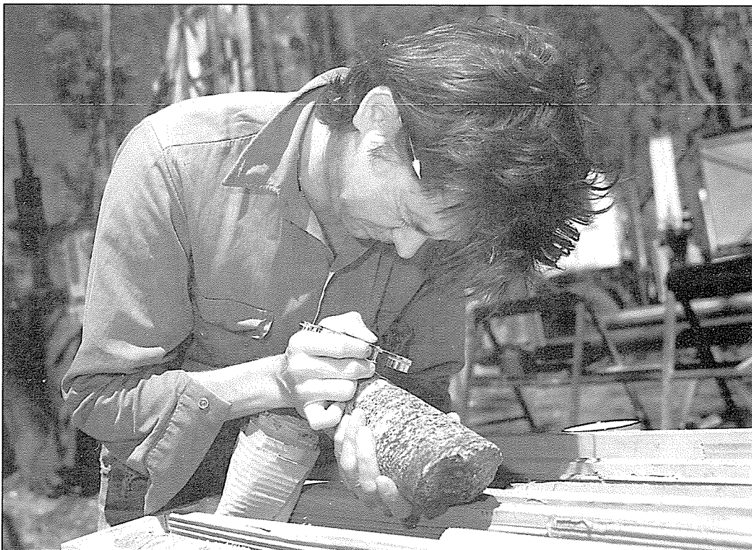
Engineering geologist Stephan Kent logging samples during site investigations for a proposed new dam in the North Dandalup area.
