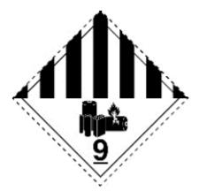
Figure 3 Class 9 label, model 9A for lithium batteries
