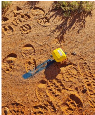
Seismic survey: a) Vibrator trucks with traffic control; b) a geophone in position; c) downloading data and recharging geophones. Photos: HiSeis Pty Ltd.
