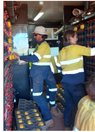
Seismic survey: a) Vibrator trucks with traffic control; b) a geophone in position; c) downloading data and recharging geophones. Photos: HiSeis Pty Ltd.
