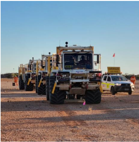
Seismic survey: a) Vibrator trucks with traffic control; b) a geophone in position; c) downloading data and recharging geophones. Photos: HiSeis Pty Ltd.
