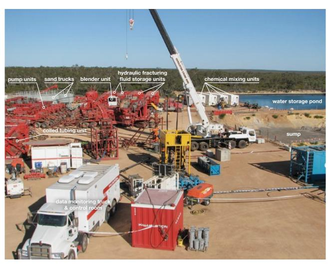
Figure 4: Hydraulic fracture stimulation equipment at the Arrowsmith 2 well site in the northern Perth Basin (courtesy of Norwest Energy Ltd)
