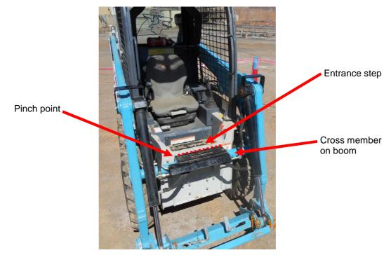
Example of skid steer involved in both incidents showing line of pinch point between entrance step and cross member on boom.
