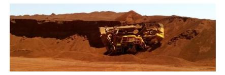
• A dozer was pushing material over an edge to create an access ramp to the pit floor when the rill of material below the dozer slumped. Mud at the bottom of the rill was pushed out, creating a circular slip failure of the slope. The dozer slid over the edge. It remained upright and stopped about half way down the slope with its blade facing down.
