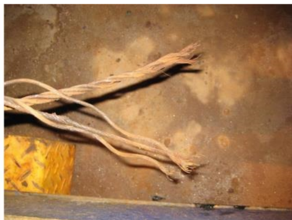
(L) Example showing a four-post hoist with failed equaliser cable. (R) Example of a failed equaliser cable.
