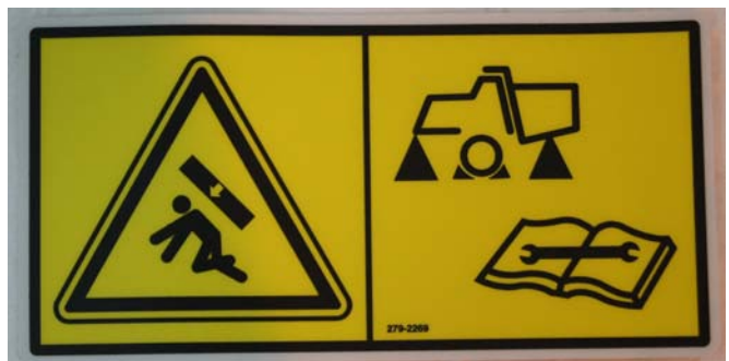
Decal warns of (a) crush hazard and (b) requirement to support vehicle and consult OEM manual before maintenance
