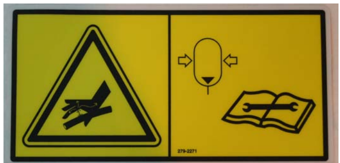
Warning label specific to stored energy hazards. Decal warns of (a) high-pressure hazard and (b) requirement to release pressure and consult OEM manual before maintenance
