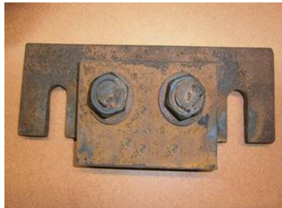
Photographs showing rail clamp as designed by OEM (left) and modified rail clamp (right) with open-ended slots and welded nuts and bolts.
