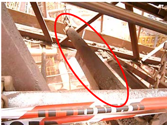
Photographs showing calibration weight requiring cleaning (left) and nearby return roller (right)
