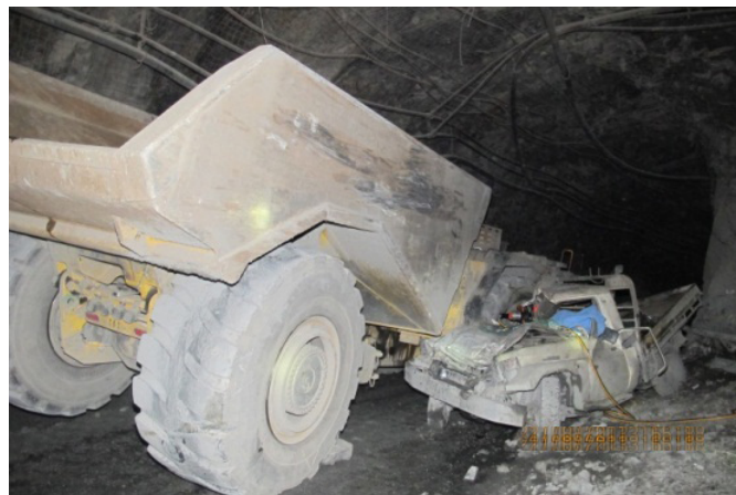
Figure 1 Incident scene after the light vehicle driver had been extracted and the truck reversed back
