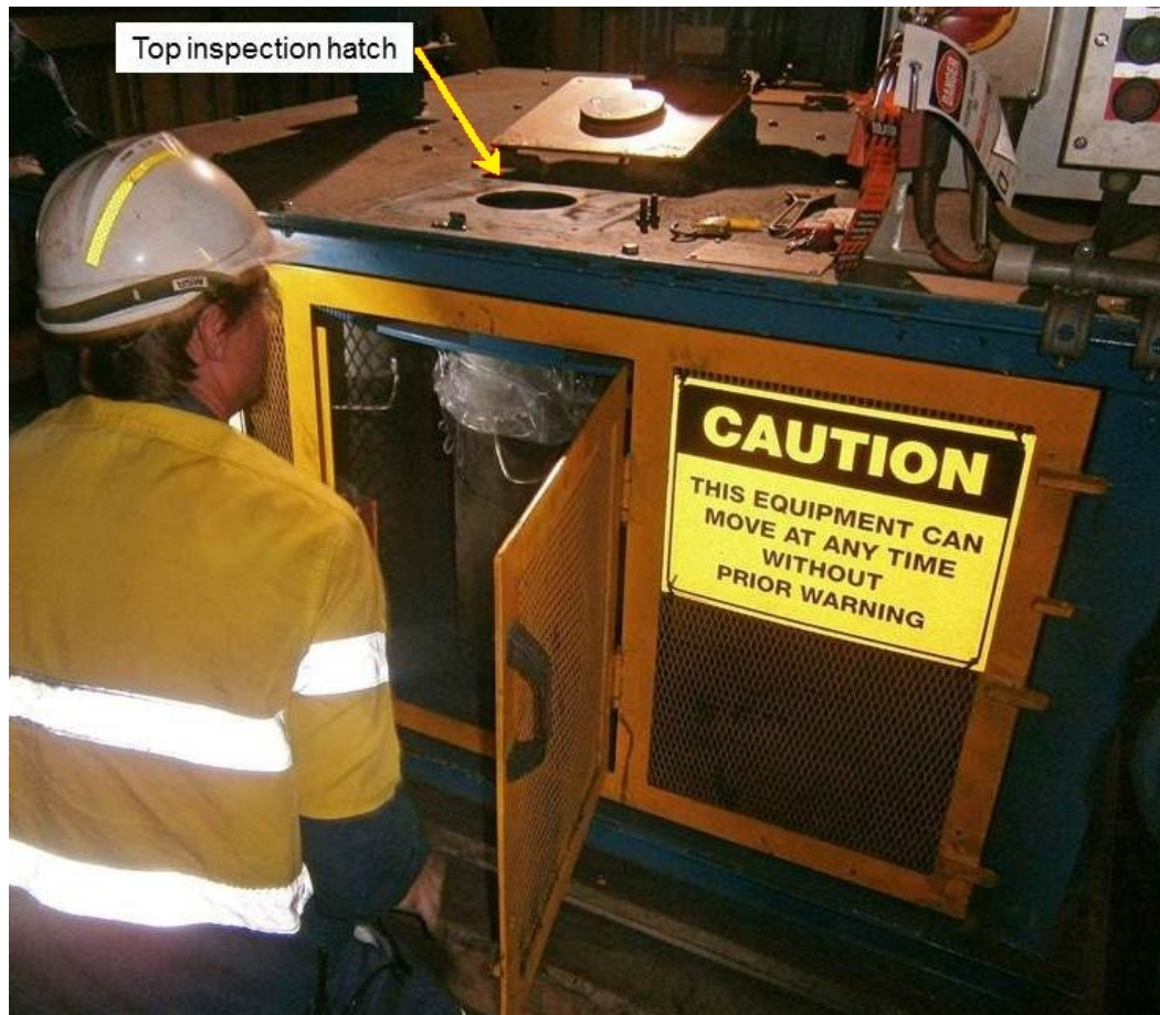
Example of 12-canister automatic rotary sample collector showing the top inspection hatch
