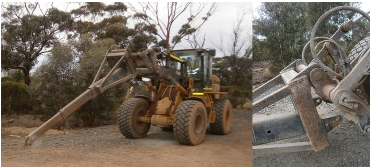
Left: IT with jib angled down. Right: Jib attachment with locking pins not engaged.
