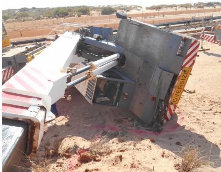
Pick-and-carry crane on its side
