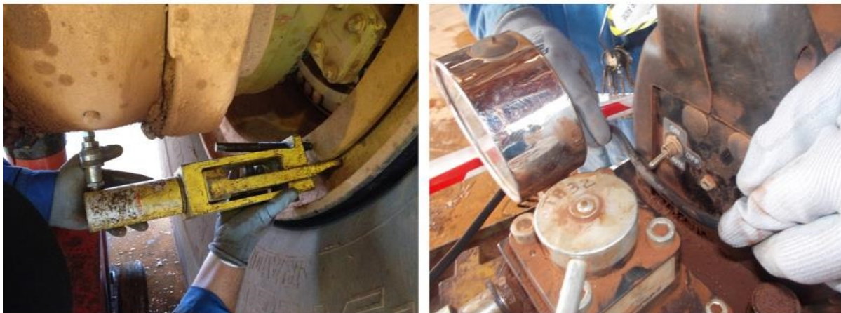
Re-enactments showing approximate hand grip on the bead breaker and position of power cable under the toggle switch
