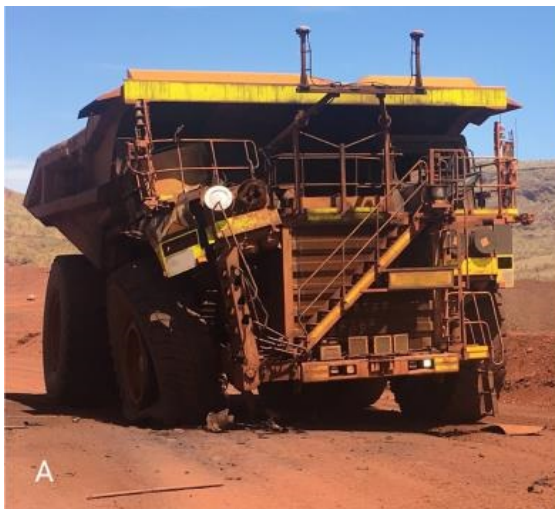
Autonomous truck struck by lightning. A. Exterior and structural damage. B. Extensive damage to deck and associated equipment. C. Interior of truck's cabin.
