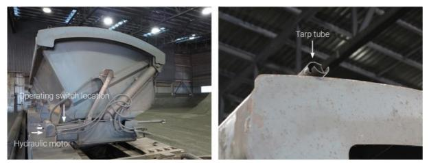
L. Detached motor and swing arm from the tarp tube. R. Fractured end of tarp tube where motor and swing arm attach on tarpaulin covering system
