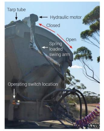
Road train trailer with swing arm attached to the tarp tube
