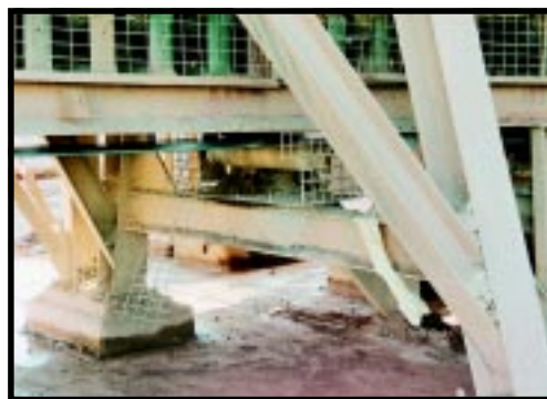
Fig (3) Clearing of spillage from around idler roller guards has always been a problem, and to cut and destroy the very purpose of a guard while allowing the spillage to remain is like waiting and priming a rat trap ready to strike. This is a contravention of Section 10(2)(c) of the Mines Safety and Inspection Act 1994.
