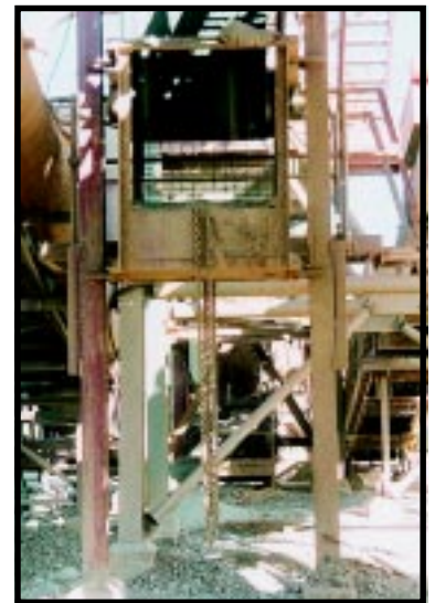
Fig (3) Clearing of spillage from around idler roller guards has always been a problem, and to cut and destroy the very purpose of a guard while allowing the spillage to remain is like waiting and priming a rat trap ready to strike. This is a contravention of Section 10(2)(c) of the Mines Safety and Inspection Act 1994.
