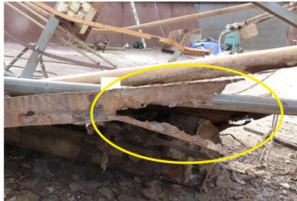
Left. Gantry bridge that failed and collapsed onto the thickener floor. Right. Corroded structural steel angle.
