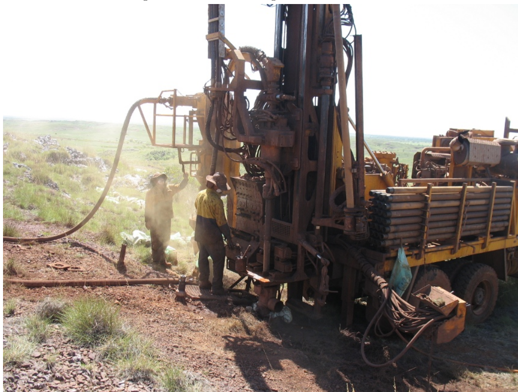
RC drilling with water injection and dust controls in place
