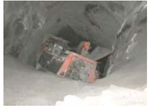
LHD 17m down an ore pass in Tara lead/zinc mine
