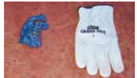
Metal fragments believed to have struck lance operator
