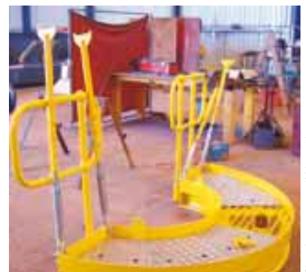
Lancing platform developed after crusher incident
