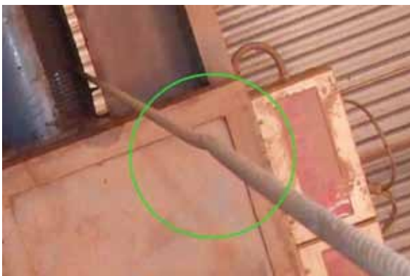
Figure 4 Kink in wire rope
