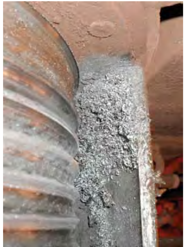
Figure 5 Rope guide shavings
