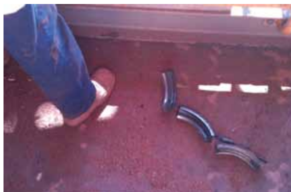
Figure 2 Final resting position of 7 kg section of rope guide and location of the employee involved in the near-miss incident
