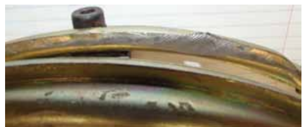
Figure 6 Wire rope imprint
