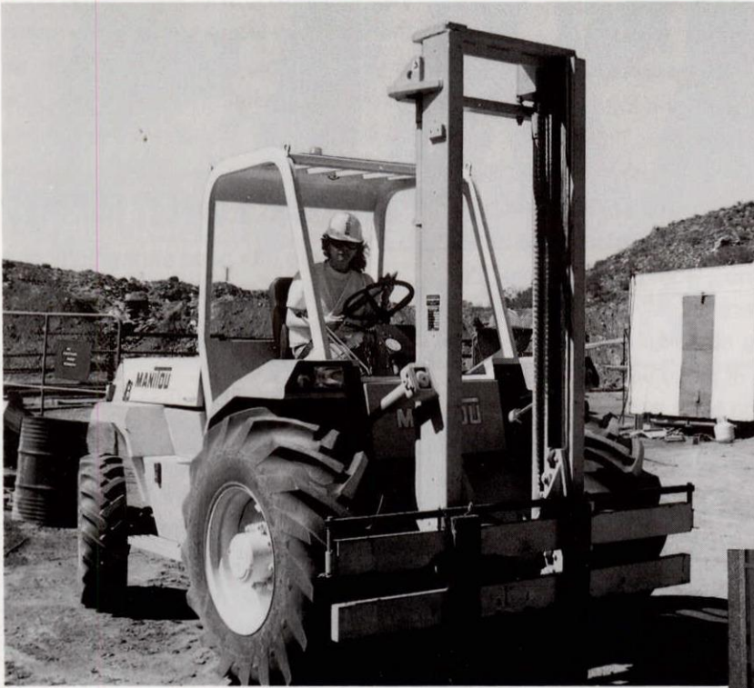
↑ Horseshoe Lights F.O.P.S canopy, seat belt and a wide based all terrain forklift for stability on uneven ground.
