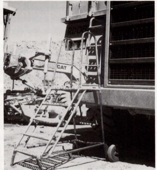
Peak Hill ↑ Access ladder for tradesman makes the job safer. ← Pulley system for leach tank covers controls lifting and saves backs.
