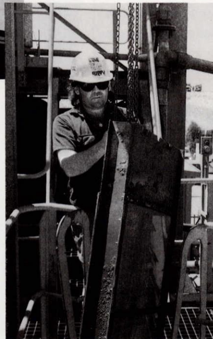
Peak Hill ↑ Access ladder for tradesman makes the job safer. ← Pulley system for leach tank covers controls lifting and saves backs.
