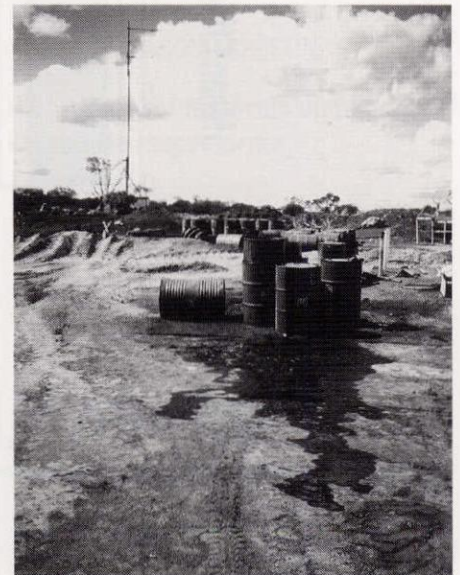
Poor storage of oil drums.
