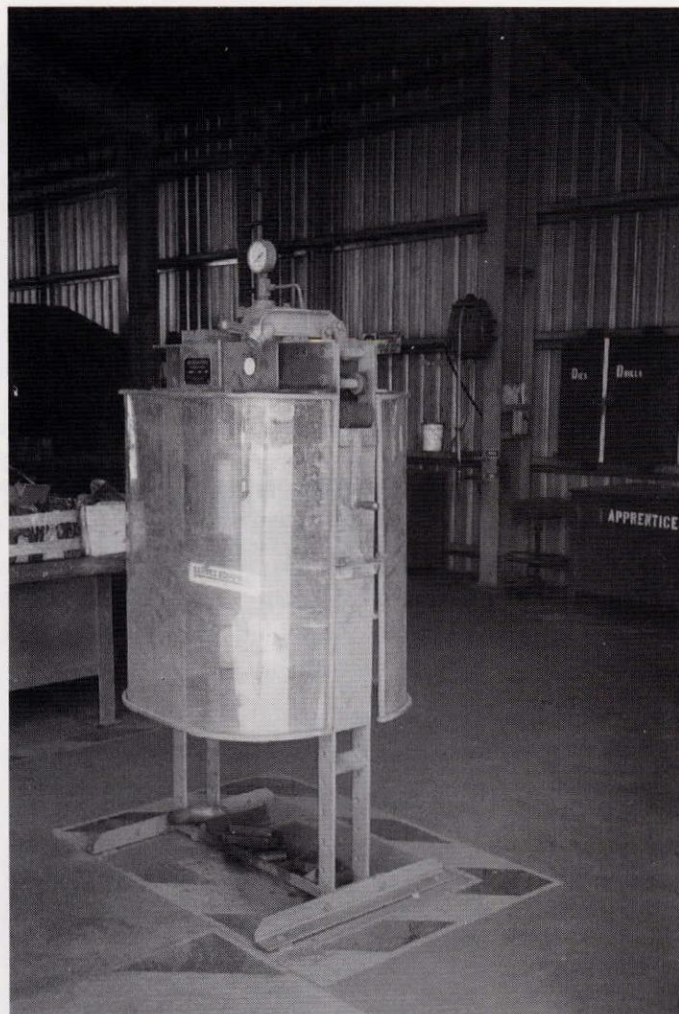
Innovative guard for hydraulic press.
