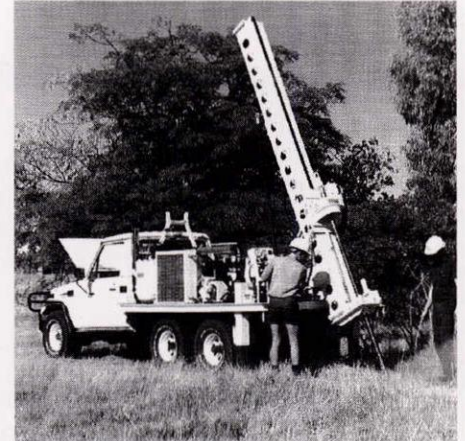
The drill rod and other moving parts should be guarded.
