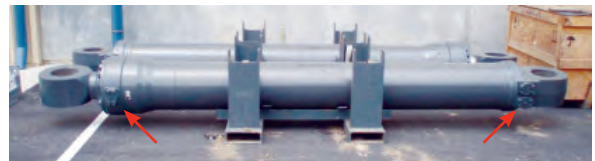
Figure 1 Location of blanking plates on tilt cylinder. Photograph courtesy of Liebherr
