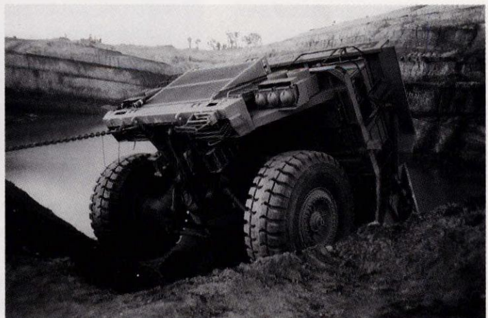
Dumping short on a wet dump requires a system to be in place that avoids any likelihood of incidents like this happening.
