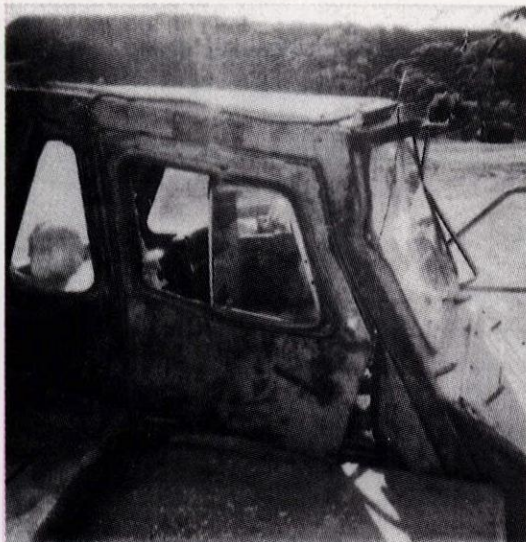
A dump truck operator was lucky to escape serious injury after running into the rear of an empty truck parked in a passing bay, waiting for a loaded truck to come up the ramp. The operator did not wait at the top of the haul ramp - a procedure that would have avoided the accident.
