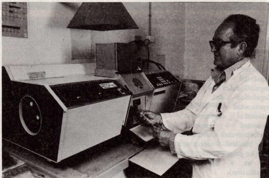
STEVE MOUNA - CHEMISTRY CENTRE LABORATORY TECHNICIAN OPERATING AN ATOMIC ABSORPTION SPECTROMETER
