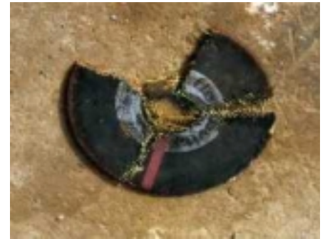
Remains of fractured grinding wheel
