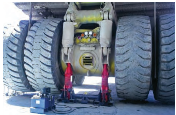
Example of fit-for-purpose jack that can be raised and locked in position to support earthmoving equipment
