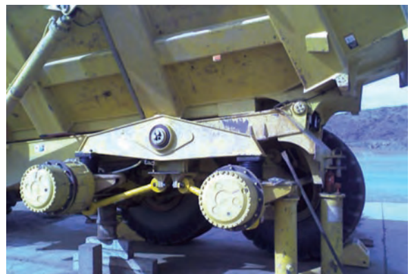
Example of inappropriate use of wooden blocks to support earthmoving equipment
