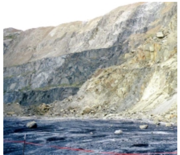
An example where large rocks have rolled 20m from the base of a pit wall.
