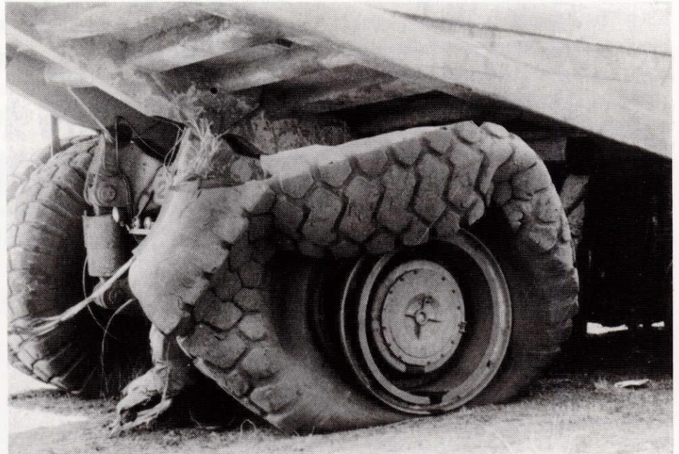
Tyre Damage caused by explosion
