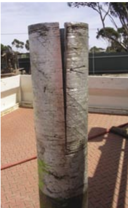
Significant Incident Report No. 135 — a side view of the split in the aluminium drill rod
