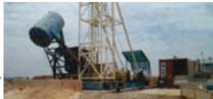
Headframe in position over shaft at Giants Reef Mining Ltd's Chariot gold project, with vacuum ore lift in place
