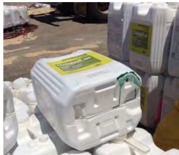
Unapproved containers damaged during the transport of dangerous goods
