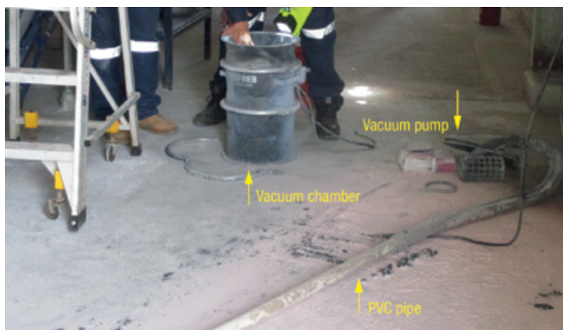
Damage to transfer system. Left. Vacuum pump chamber and pump, PVC transfer piping and evidence of spot fires on the floor. Right. Distortion of hopper caused by explosion
