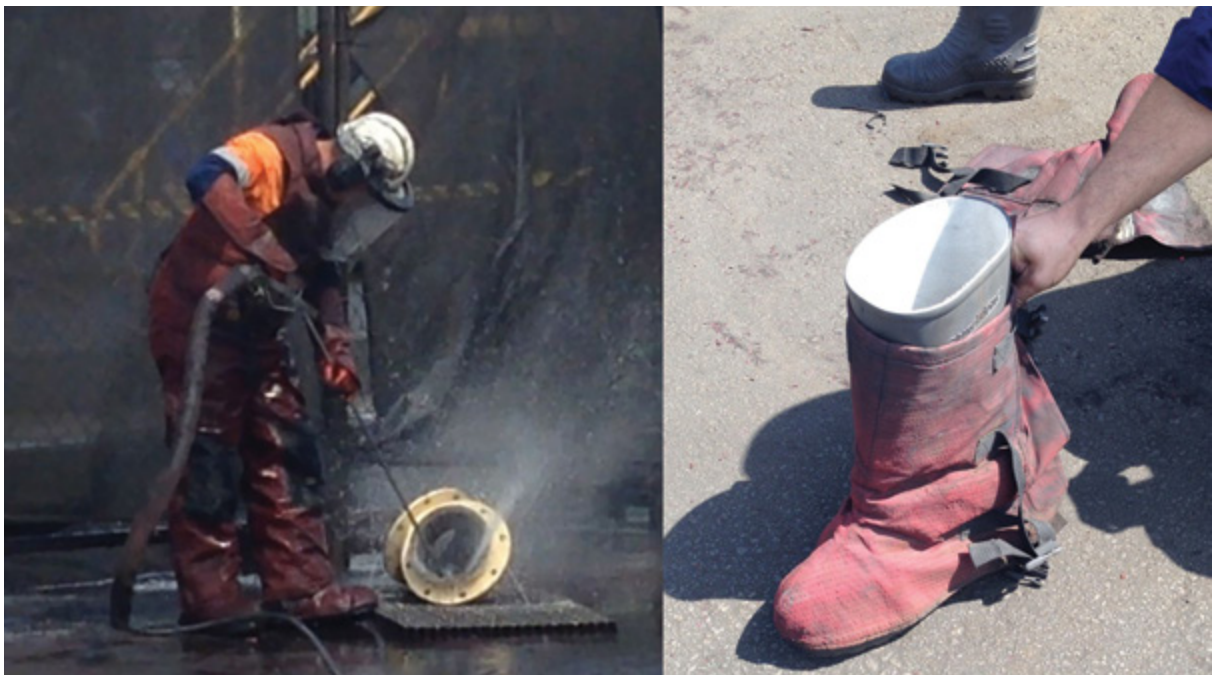
Personal protective equipment. Left: Worker using high-pressure water jetting equipment while wearing appropriate face shield, blast suit, protective gloves, and boots with covering foot shield. Right: Protective boot and covering foot shield
