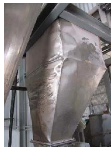
Damage to transfer system. Left. Vacuum pump chamber and pump, PVC transfer piping and evidence of spot fires on the floor. Right. Distortion of hopper caused by explosion
