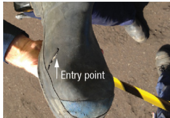
Entry point where high-pressure water jet penetrated boot lining
