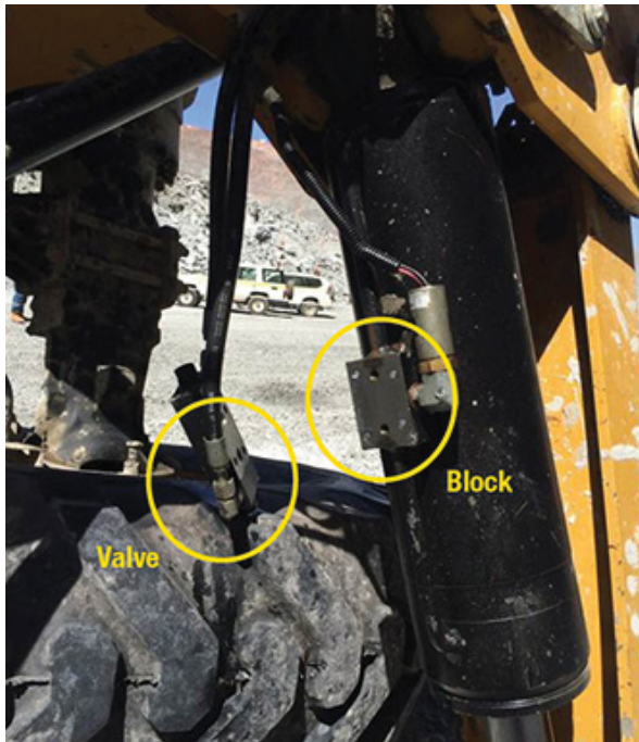
Damaged check valve block. Left: Check valve separated from block. Right: Sheared bolts on check valve block
