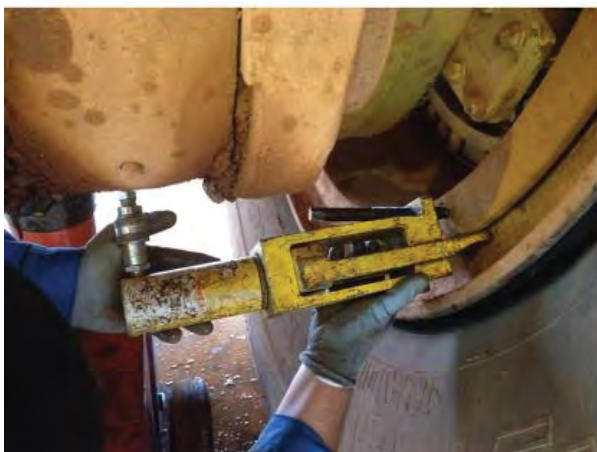
Re-enactments showing approximate hand grip on the bead breaker and position of power cable under the toggle switch
