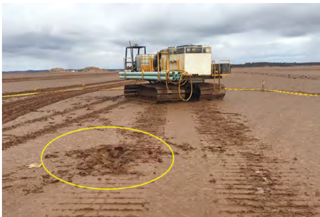
Left: Vehicle track marks and indentation where the offsider was pushed into the soft ground. Right: Straps used to hold both control levers in the forward moving position.
