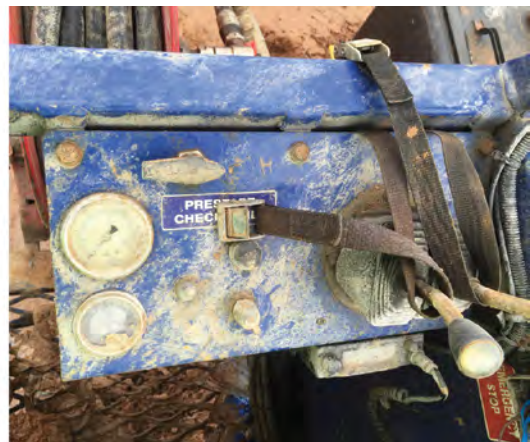
Left: Vehicle track marks and indentation where the offsider was pushed into the soft ground. Right: Straps used to hold both control levers in the forward moving position.
