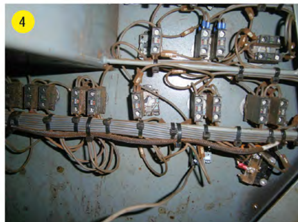
1. Bent head-slide bracket shown with drill head above the deck wrench 2. New head slide did not fit between head bracket and mast 3. Driller's cabin showing seat position and control panel 4. Exposed wires and switches on the underside of the control panel.
