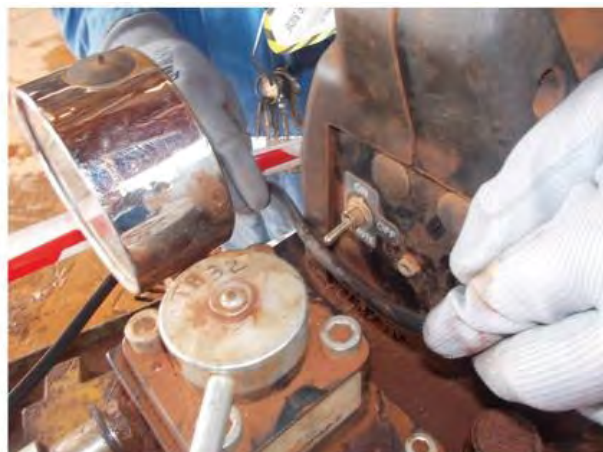
Re-enactments showing approximate hand grip on the bead breaker and position of power cable under the toggle switch
