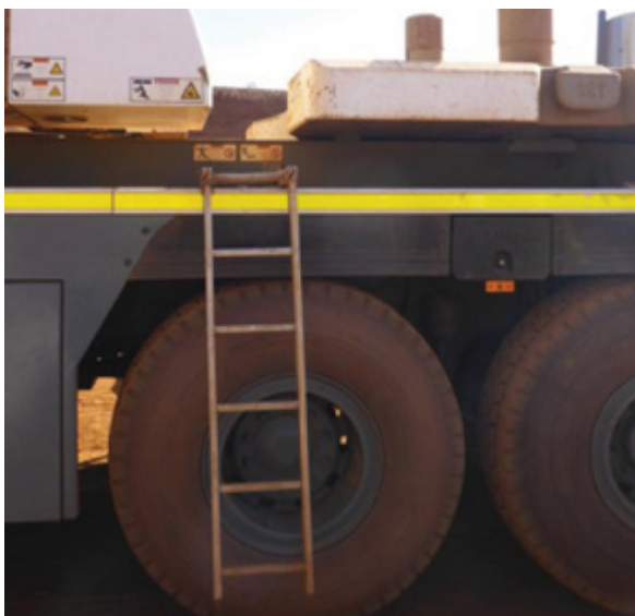
The ladder used to access the crane deck
