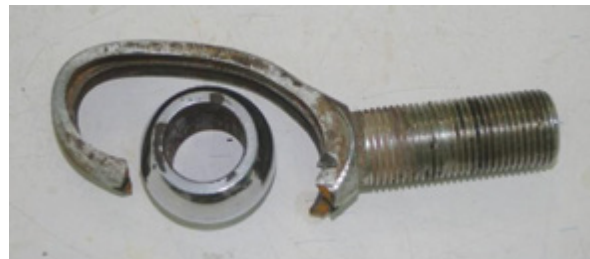
Damaged steering tie rod coupling from the EWP
