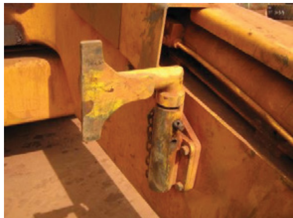
Example of fall-back arrester arm showing components that can become projectiles
