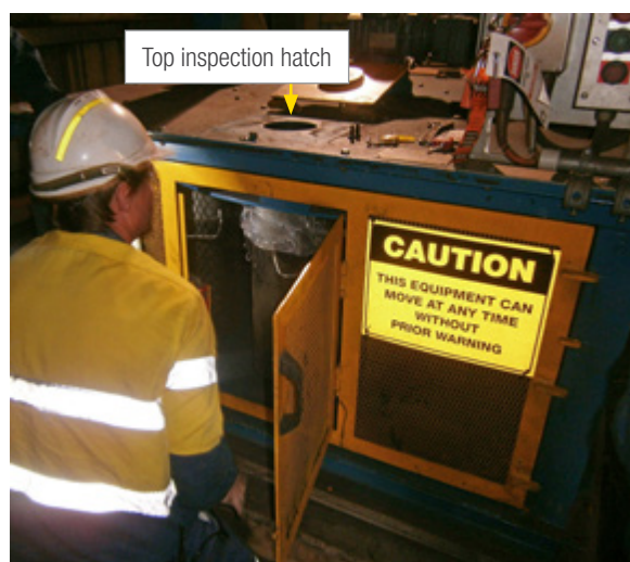
Example of 12-canister automatic rotary sample collector showing the top inspection hatch
