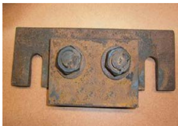
Photographs showing rail clamp as designed by OEM (top) and modified rail clamp (bottom) with open-ended slots and welded nuts and bolts
