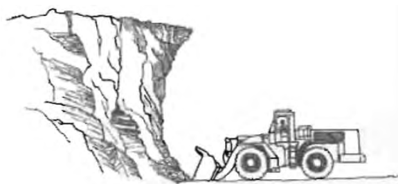
An undercut face showing overhang (diagram from Mine Safety and Health Administration, 2001)
